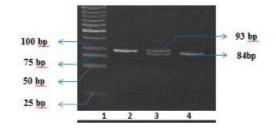
Del site in exon 1 of the APOB gene was analysed by amplifying a fragment of 93/84 bp using two primers designed by Boerwinkle et al. (18)5'-• CAGCTGGCGATGGACCCGCCGA-5'-3' (forward primer) and ACCGGCCCTGGCGCCCGCCAGCA-3' (reverse primer).
